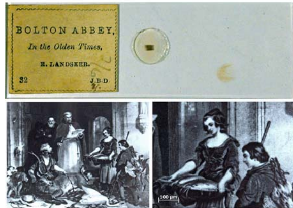
Figure 1) Upper image of a J. B. Dancer microphotograph slide. The slide is a standard 1" by 3" glass slide and the microphotograph on the slide measures 1.8 mm by 1.4 mm. Lower left is a photomicrograph of the microphotograph. The lower right image shows a portion of the microphotograph with a scale inserted.
